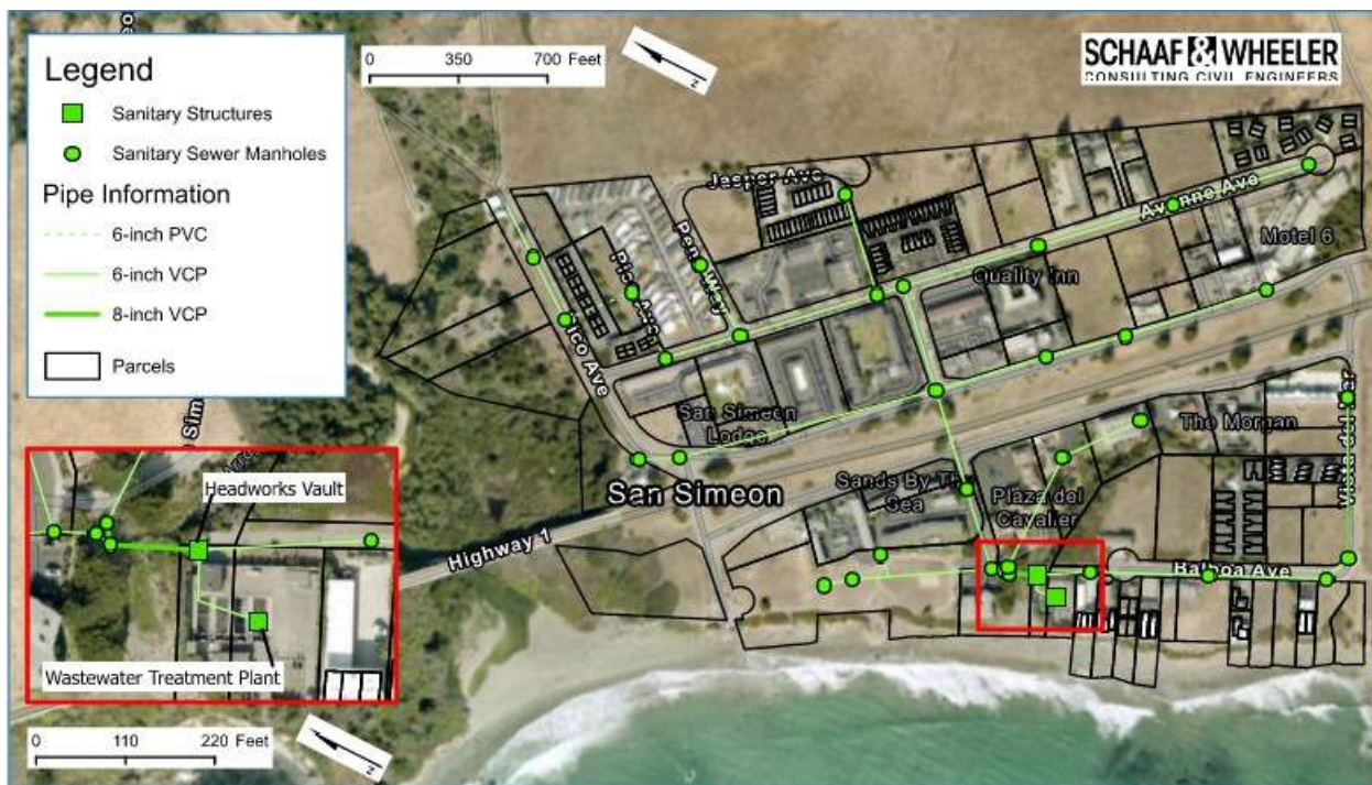
Figure 3. SSCSD Sewer System Overview
