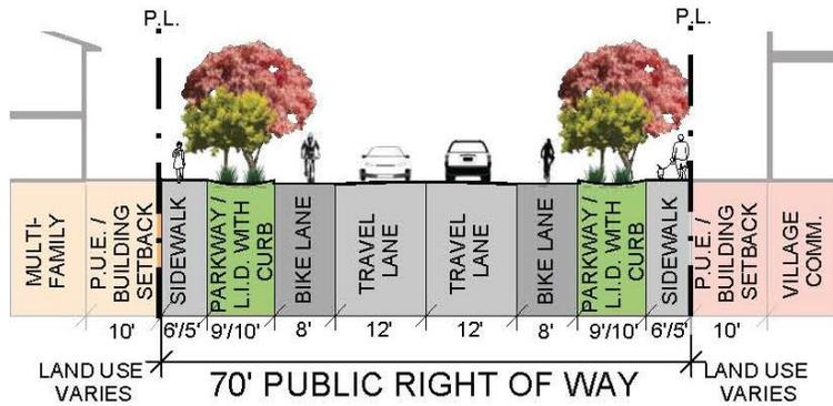
NOTE: DETACHED SIDEWALK WIDTH FOR COMMERCIAL RETAIL SHALL BE 6'-0", FOR ALL OTHER LAND USES, SIDEWALK MAY REDUCE TO 5'-0" AND L.I.D. WOULD WIDEN TO 10'-0"
