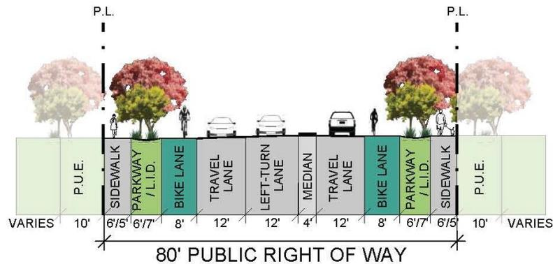
NOTE: DETACHED SIDEWALK WIDTH FOR COMMERCIAL RETAIL SHALL BE 6'-0", FOR ALL OTHER LAND USES, SIDEWALK MAY REDUCE TO 5'-0" AND L.I.D. WOULD WIDEN TO 8'-0"
